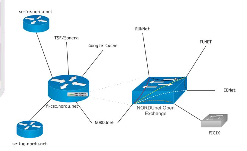
Ethernet switching fabric, with (potential) MPLS and OpenFlow capabilities, adjacent to routing capability
