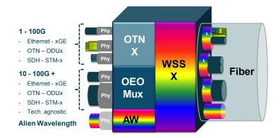
Figure 5.4: Integrated digital OTN switching or grooming using ODUFlex
