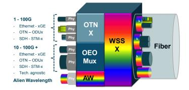
Figure 6.1: Integrated digital OTN switching or grooming using ODUFlex
