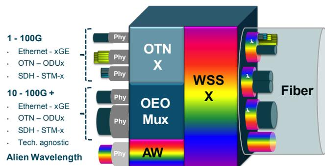
Figure 6.1: Integrated digital OTN switching or grooming using ODUFlex
