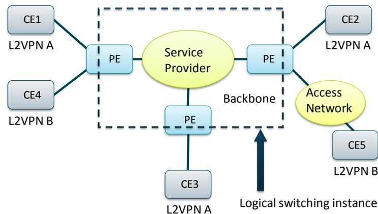
Figure 5.5: Reference model for L2VPNs (source: [RFC4665])
