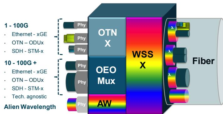
Figure 5.4: Integrated digital OTN switching or grooming using ODUFlex
