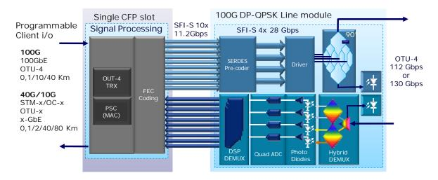
Figure 4-5: OIF system reference model based on a 100G scenario.
