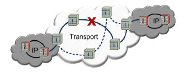
Figure 6-1: Dual IP domains interconnect via GMPLS enabled Transport layer providing protection.
